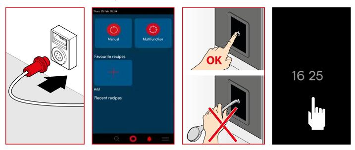
To switch on the equipment, insert the plug into the dedicated socket. After a few moments the main page will appear. It is recommended to only use your fingers to touch the touch screen, avoiding the use of tools (e.g. forks, ladles, etc.). After several minutes of disuse, the keyboard automatically locks to prevent the cycle in progress from being accidentally stopped. To unlock the keyboard, touch the display.
