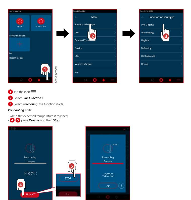
6 When *Precooling* has been completed, the "*completed*" message appears. After reaching the pre-cooling temperature, the equipment maintains the temperature until the door is opened.
