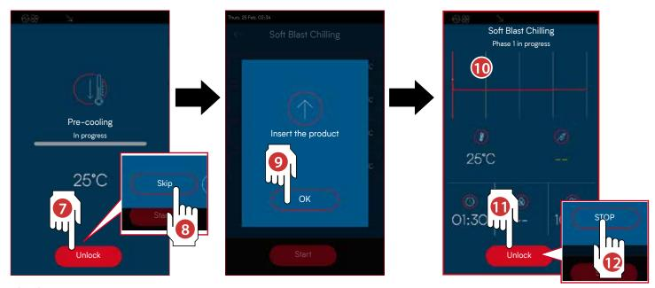
7 8 After touching Start, an automatic variable duration precooling of the chamber starts. If this is not required, press the **Release** button and then **Skip**.
