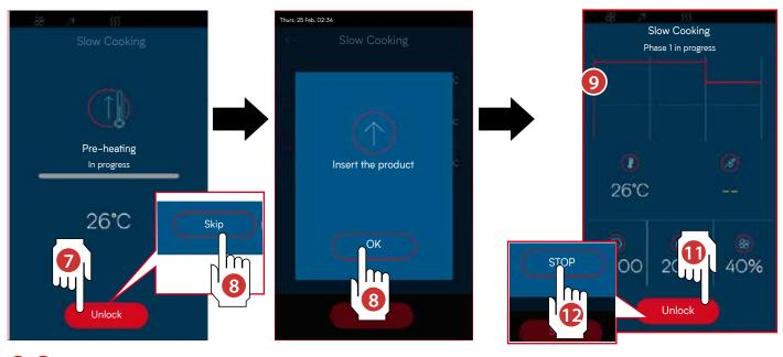
7 8 After touching *Start*, an automatic variable duration preheating of the chamber starts. If this is not required, press the *Release* button and then *Skip*.
