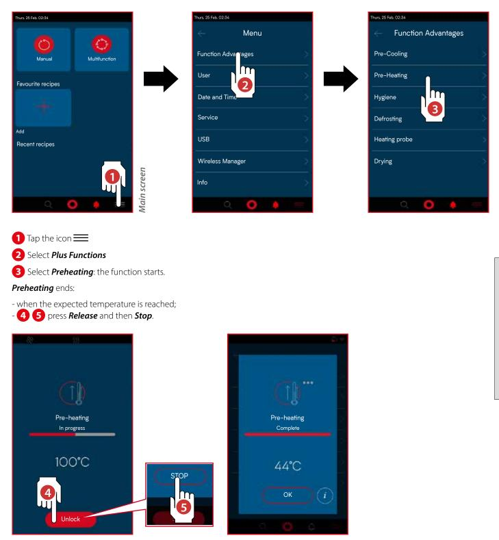
6 When **Preheating** has been completed, the "**completed**" message appears. After reaching the pre-cooling temperature, the equipment maintains the temperature until the door is opened.
