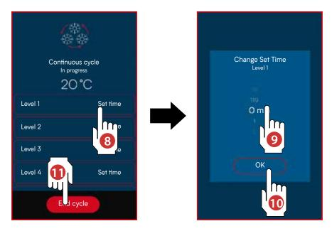
8 9 10 Set the desired time in minutes for each tray (level) (e.g. from 0 to 119 minutes). Confirm the entered time with "OK". The countdown of each timer set for each tray begins; when a timer expires, an acoustic signal sounds and a screen indicates which tray to remove.
