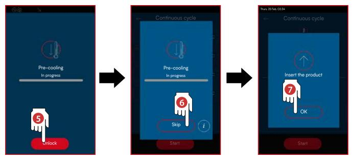
5 6 After touching Start, an automatic variable duration precooling of the chamber starts. If this is not required, press the Release button and then Skip.
