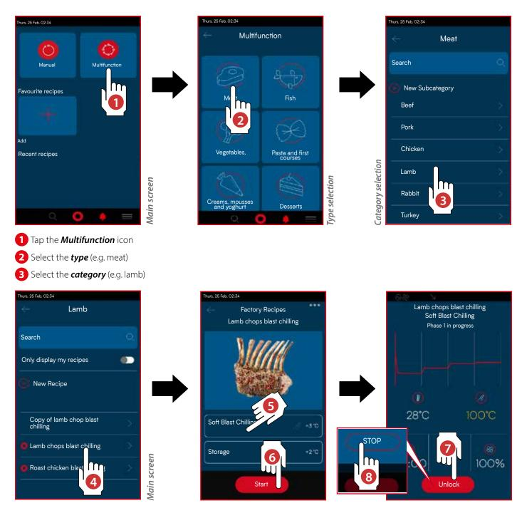
4 Select the *recipe* to be started (e.g. Blast chilling of lamb ribs); to facilitate the search, it is possible to filter the recipes by viewing only the user's personal recipes. The recipes preceded by the symbol are factory pre-set recipes: they cannot be renamed or deleted.
