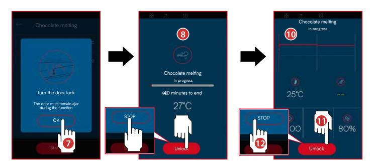
7 After tapping the word **Start** a screen warns that the door must remain ajar, by turning the door lock.
